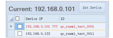
Fig. 3-13 RAEM1 Configuration Tool Device Offline
