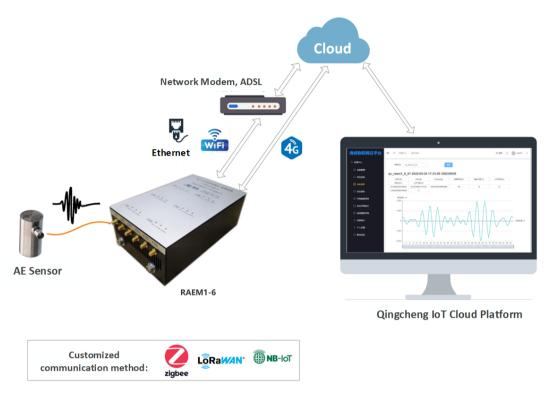
Figure 4-1 Connecting the RAEM1-6 monitoring system
