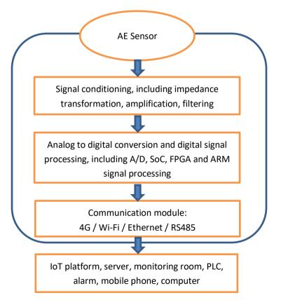
Fig. 2-2 RAEM1 Functional modules flow diagram
