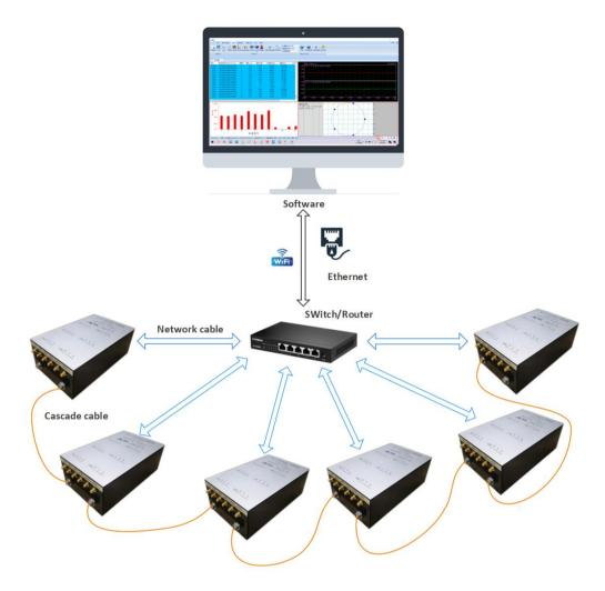
Fig. 3-8 Wi-Fi networking for RAEM1-6 desktop monitor
