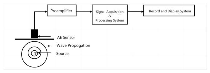
Fig. 1-1 Block diagram of acoustic emission testing principle
