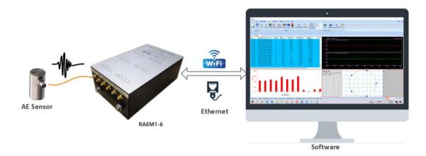
Fig. 3-1 Connection diagram of RAEM1-6 desktop detector
