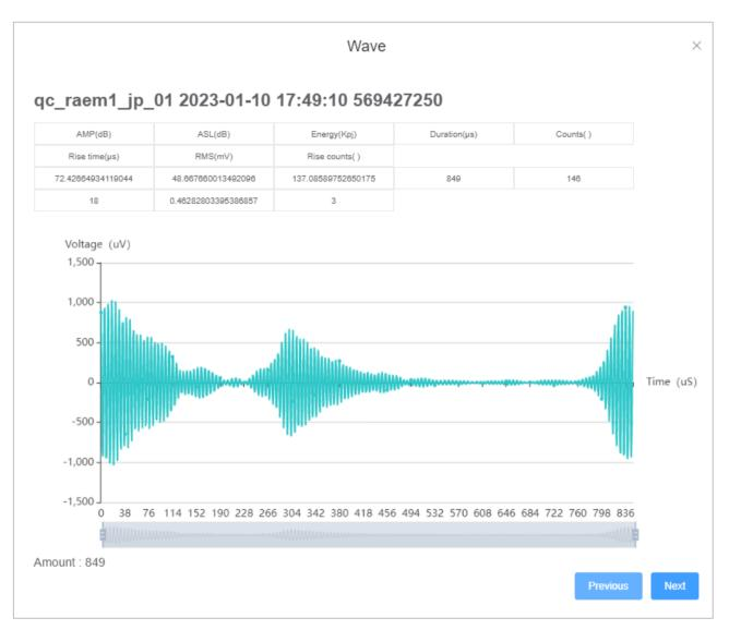
Fig. 4-18 Waveform page from the Data monitoring
