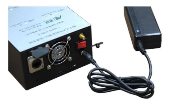
Fig. 2-7 Hardware connection of RAEM1-6 - Rear
