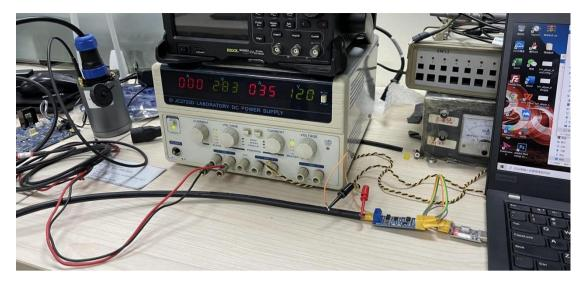
Fig. 7-8 RAEM1 485 hardware test setup
