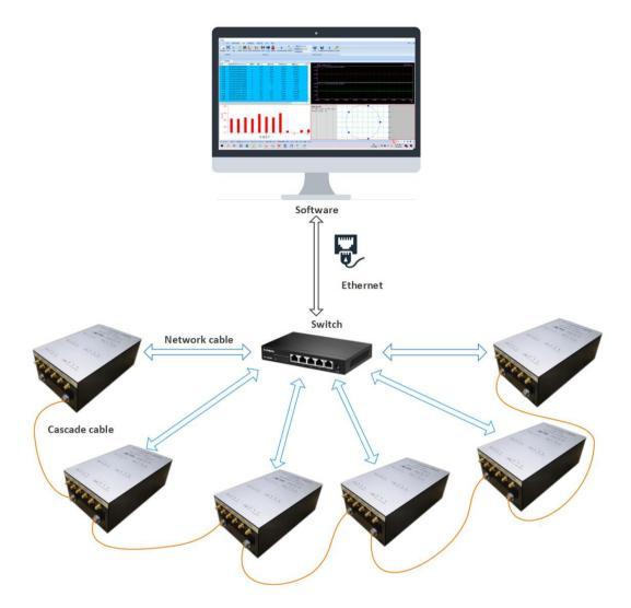
Fig. 3-3 Network connection of a RAEM1-6 desktop monitor
