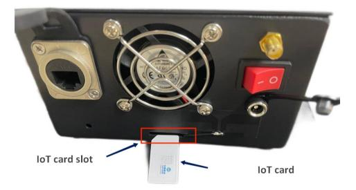
Fig. 4-3 RAEM1-6 Network adapter and card slot for the Internet of Things
